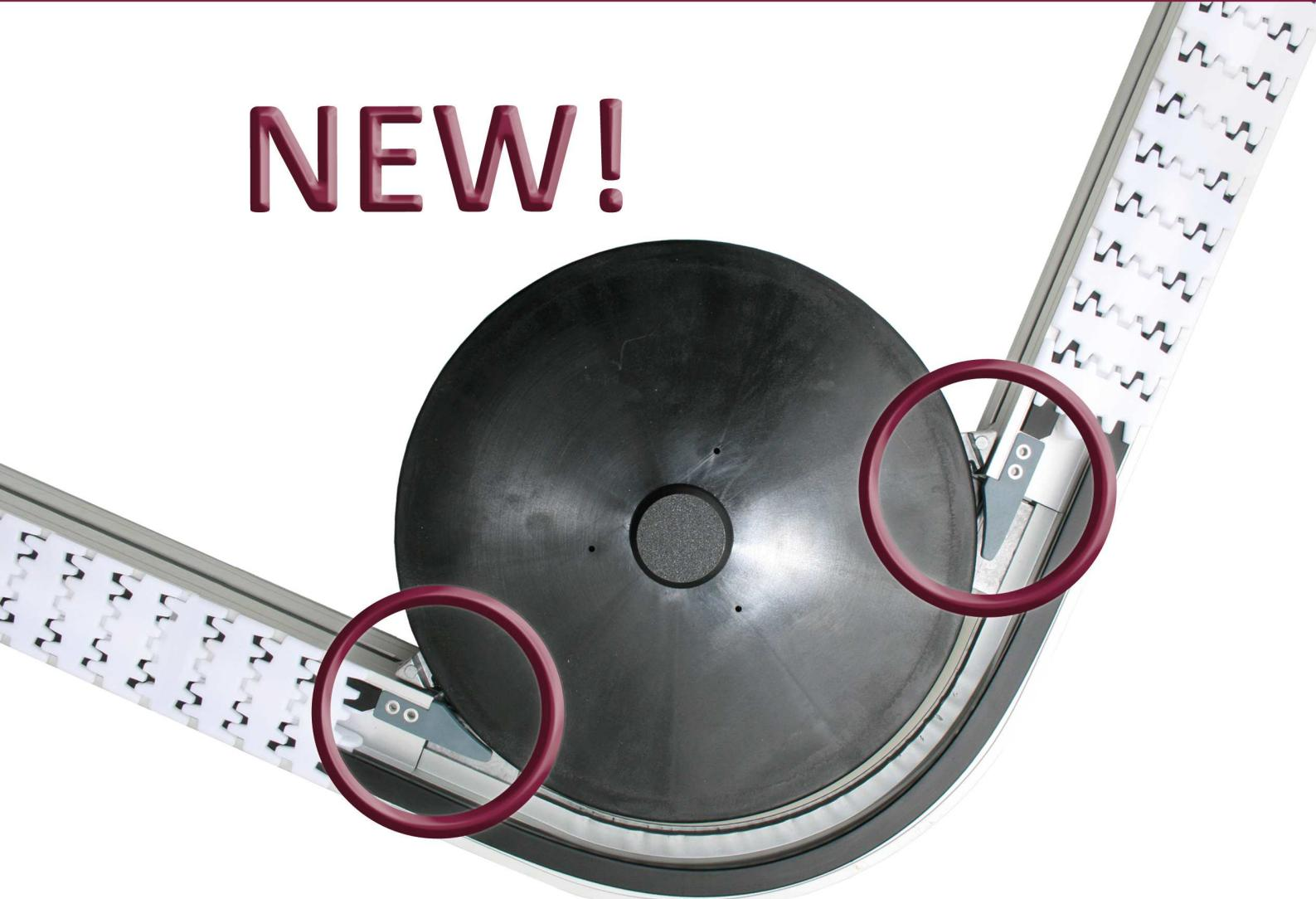
Improved installation of sliderails at plastic chain
